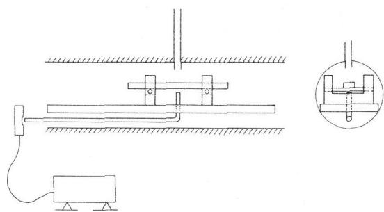
FIG. 3. Another test arrangement using a steel wave guide to transmit the acoustic vibrations from the specimen to the microphone outside the furnace.
