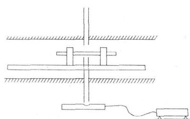
FIG. 4. The arrangement that proved to give the most reproducible results for dynamic modulus measurements at moderate temperatures with the IET. The microphone is located directly underneath the center of the specimen.
