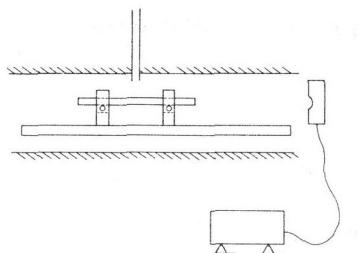
FIG. 2. The first arrangement explored for operation of the IET at moderate temperatures. The microphone is positioned on the end of the furnace tube.
