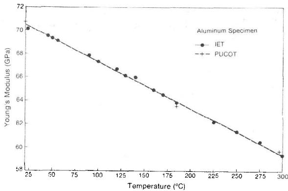
FIG. 5. Experimental data obtained with the IET and with the PUCOT (piezoelectric ultrasonic composite oscillator technique) for 99.99% pure aluminum over the temperature range 25° to 300°C.
