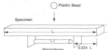
FIG. 1. The recommended setup for the operation of the impulse excitation technique (IET) at room temperature. The small projectile (such as a bead or small steel ball) causes the specimen to vibrate in the fundamental flexural mode and the microphone detects the resulting vibrations.
